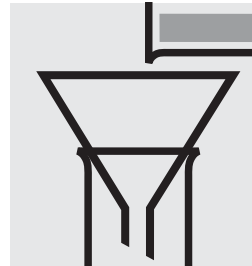
Transfer the residue to a 20-ml volumetric glass using a little distilled water.
